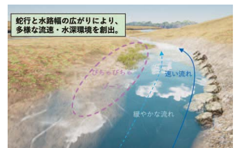
River channel drilling with consideration for the river environment (3D imagery)
