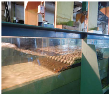
Hydraulic model experiment to confirm the effectiveness of artificial reef scouring measures
