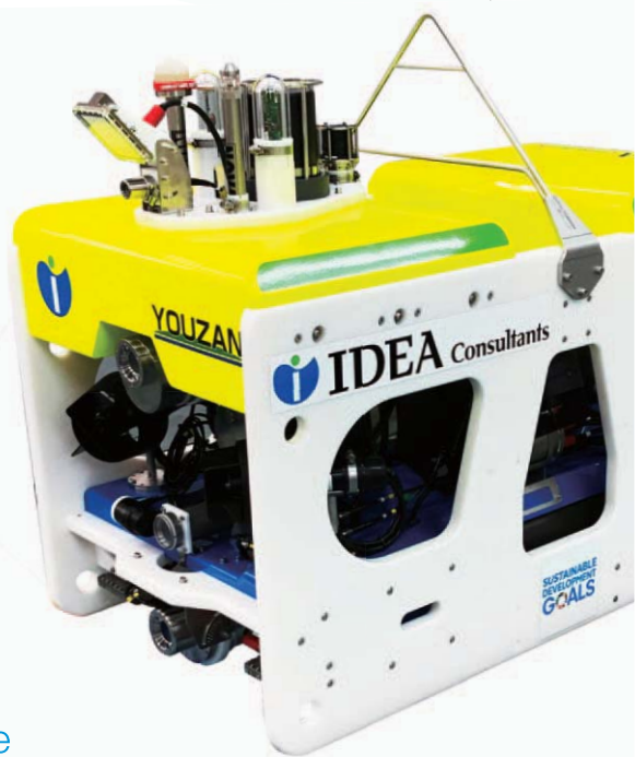
Hovering type AUV, developed in-house: YOUZAN
